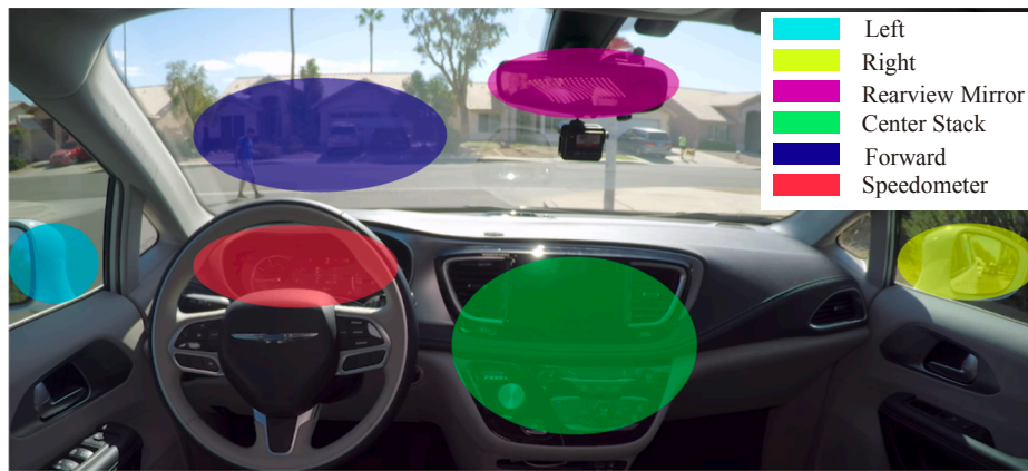
Fig. 10. Illustration of the driving assistant. Highlighted locations represent the gaze of driver.
