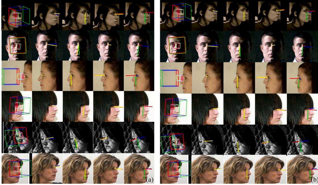
Fig. 8. (a) and (b) show the experimental results of HopeNet and ADML on the sample of AFLW2000 dataset, respectively. The first column of small cubes indicates the predicted values, the large cubes indicate the true values, the yellow line indicates the true values, and the other lines indicate the predicted values.
